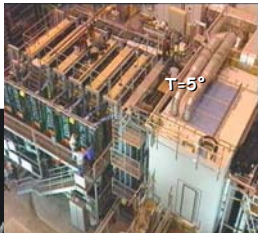
770 kg emulsion target and scintillating fibre tracker
